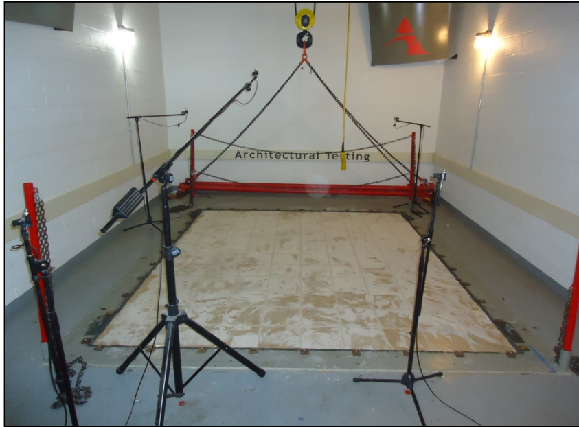
Source Room View of Test Specimen Installation
