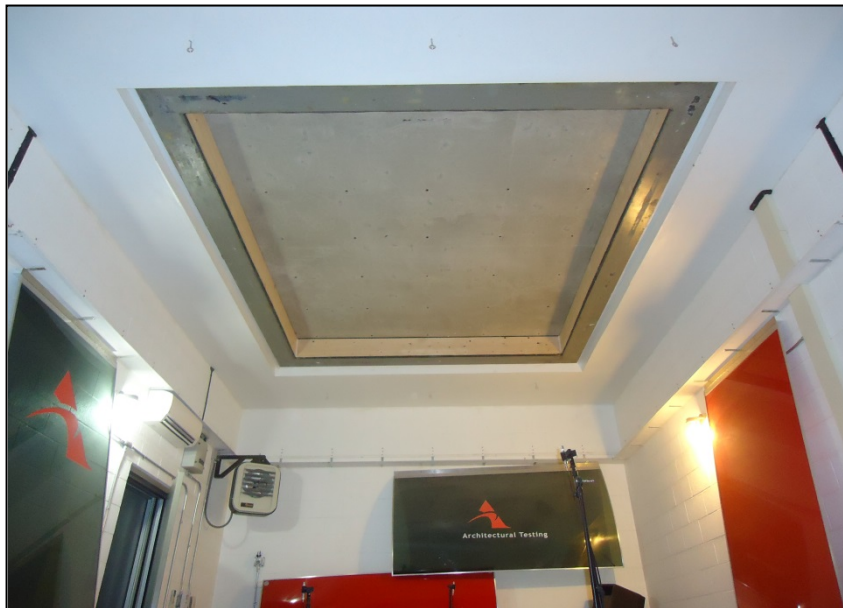
Receive Room View of Test Specimen Installation
